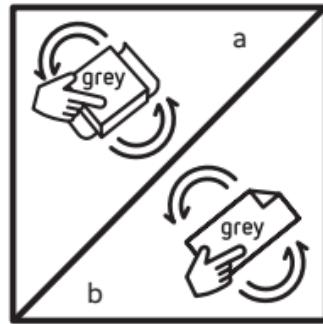
13. Place the grey paper on the block and finish the polish (a). In case of a rounded surface use only the paper, without the block (b).
