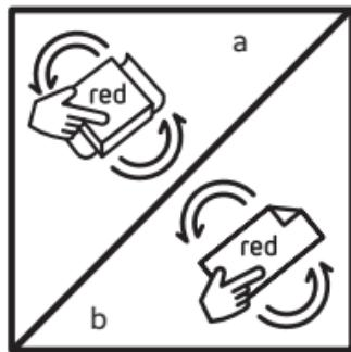
12. Place the paper on the block and use the red side to sand down the repair until the excess of the mass is removed and an even surface is obtained (a). In case of a rounded surface use the paper, without the block (b).
