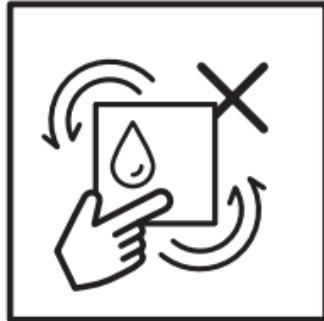
2. Wash the damaged place with a degreasing agent (e.g. acetone, alcohol).
