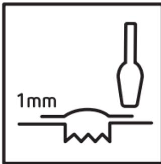
8. Place a required amount of mass until an excess of 1 mm above the material surface is obtained.
