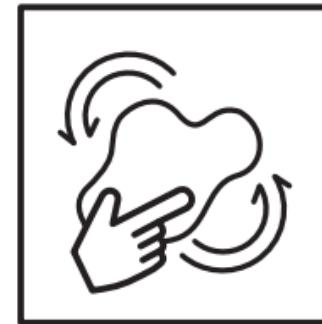
15. Place the container on a soft cloth and pressing down use circular motions to polish the repaired surface.
