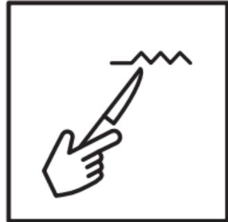
1. Clean the damaged place with a sharp tool in order to remove the remains of the Gelcoat, dust and other dirt.
