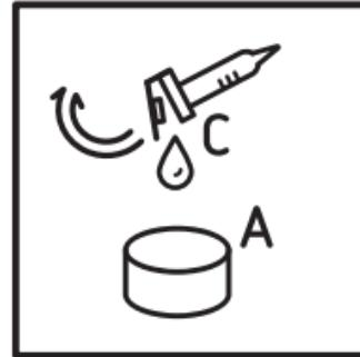
4. Open the container with the curing agent. Carefully pour its contents into the Gelcoat packaging.
